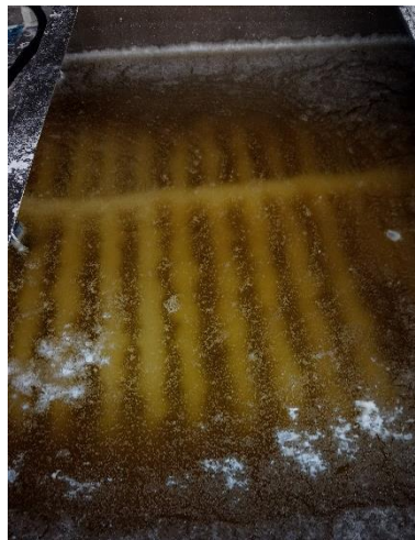
Figure 9. Molten PCM and detail of the coils. Crystallisation on the surface is evidence of the low temperatures in the area.
